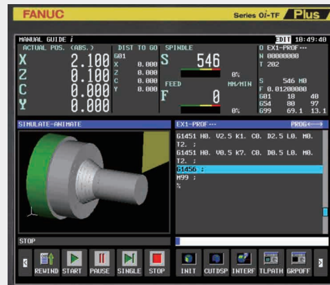
Check cutting result using cutting simulation
