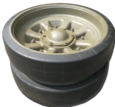
Ground wheel into the T-72 tank 172-50-053SB
